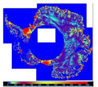
Modified Antarctic Mapping Mission (SAR interferometry) (K. Farness and K. Jezek)
